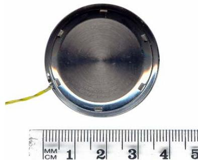
Currently our device in development, use kinetic energy from natural body movement to generate electricity.
